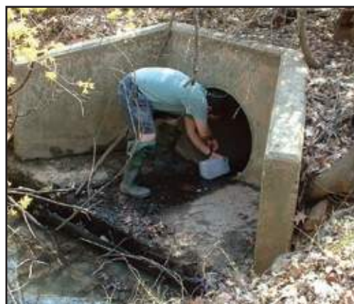
Figure 30: Measuring flow (as volume per time)
