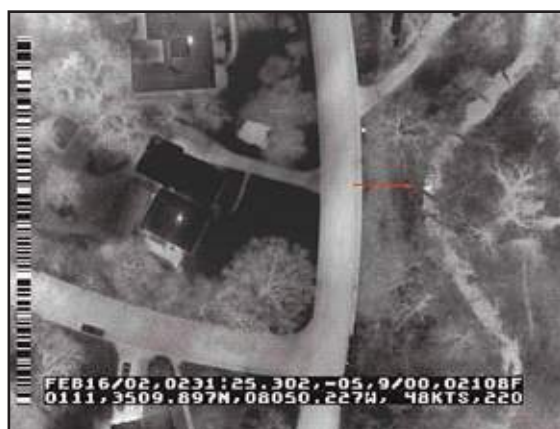
Figure 72: Aerial thermography showing sewage leak
