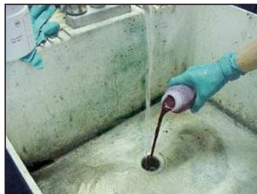
Figure 63: Dye Testing Plumbing (NEIWPCC, 2003)
