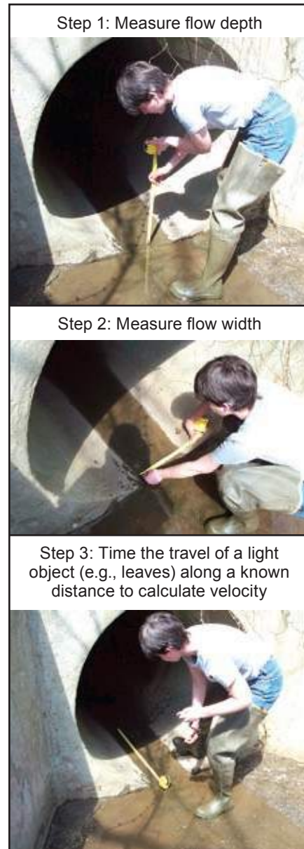
Figure 31: Measuring flow (as velocity times cross-sectional area)
