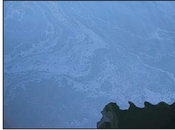
Figure 36: Synthetic versus Natural Sheen (a) Sheen from bacteria such as iron floc forms a sheet-like film that cracks if disturbed (b) Synthetic oil forms a swirling pattern
