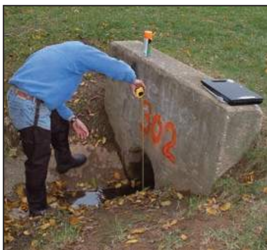
Figure 27: Measuring Outfall Diameter
